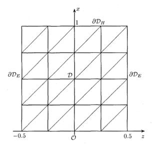
Fig. 1. Cube subdivided in bricks that in turn may be subdivided in tetrahedra or prisms, side view
