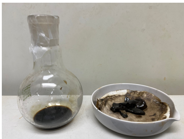
Figure 4.1: HTL of PS at 300°C, 45 minutes.
