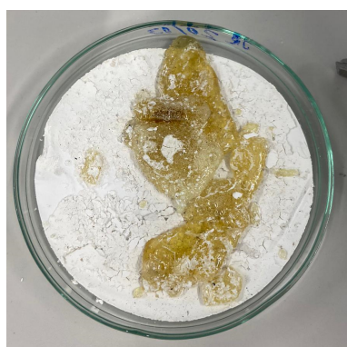
(a) Char and catalyst (Run 11, 330°C, 7.5 wt%, 30 min).
