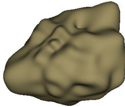
Figure 6.2 An irregular shape particle described by spherical harmonics. The particle width is 15.56 \mu\text{m} . (In this study the particle width was used as the measure of particle size, see details in the text)
