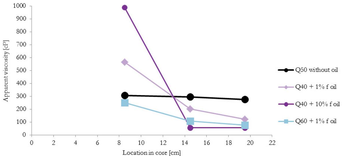
**Figure 5** Apparent viscosity of pre-generated foam with surfactant A and oil over the length of the core. Q50: 50% foam quality, etc. f: fractional flow of oil in injected fluids.
