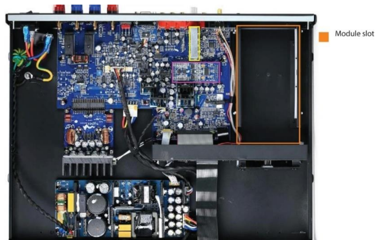
Figure 24: A double module slot, one above another, which can be installed from the back.
