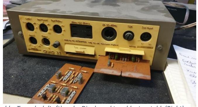
Figure 23: A Tape board to add a Tape deck (Left) and a Disc board to add a turntable(Right)
