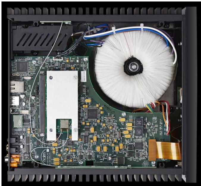
Figure 7: AiOs with 'everything' on one, complex, PCB.
