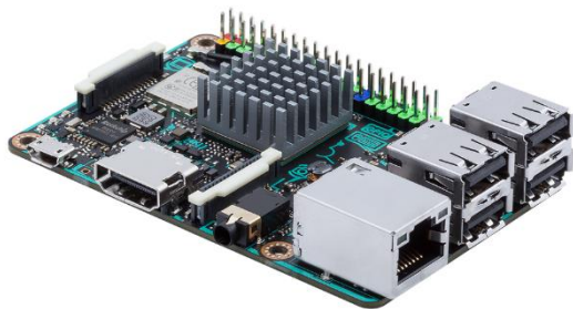
Figure 52: Asus Tinker Board: A microcomputer designed for integration and custom builds.
