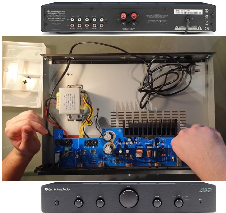
Figure 20: Opened up during disassembly, connectors at the back already removed.
