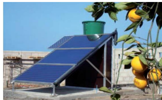
MEMBRANE DISTILLATION SYSTEM
