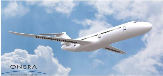
**Figure 3.1:** Illustration of the ONERA Dragon aircraft [49]. Figure shows a version with more than 13 EDFs per wing.
