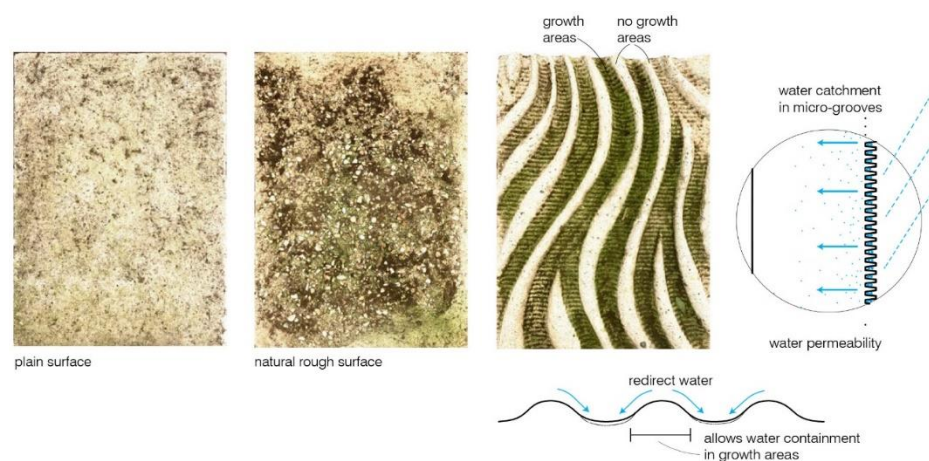
Figure 14. Geometric features to enhance bio-receptive qualities in comparison to natural surfaces.
