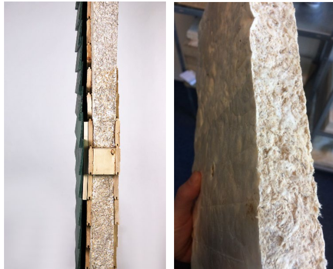
Figure 8 & 9. Insulation of Ecovativ (left) and Mogu (right). (8. Ecovative, 2018b and 9. own picture made at Fungalogic 1 )
