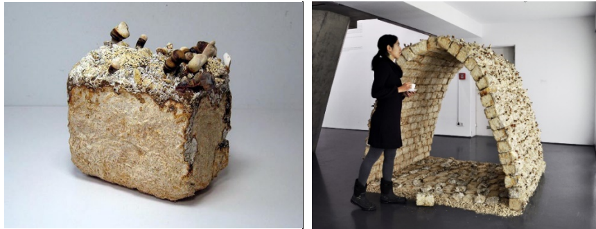
Figure 13 & 14. Mycelium brick (left) of the Alpha tea house (right) by Phillip Ross. Source: Roth-Johnson, 2014.
