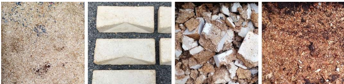
Figure 12. Mycelium bricks of the Hy-Fi tower at MoMa PS1 in New York. Source: Shaw, 2014
