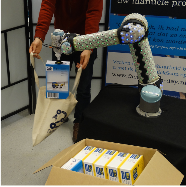
Fig. 2. Collaborative product handling robot application developed in Factory-in-a-day.
