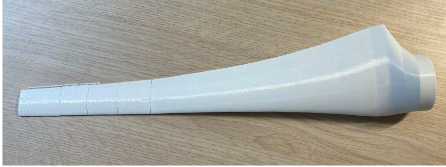
Figure 4.12: First 3D printed blade trial, broken at four different locations.
