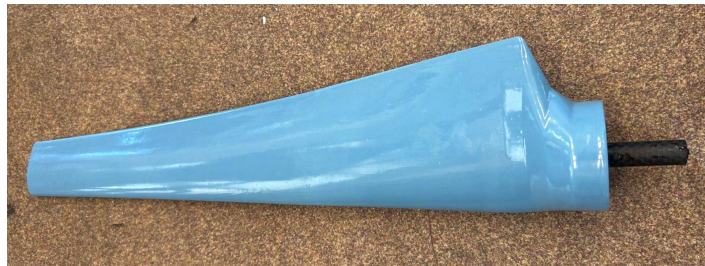
Figure 4.24: 3D printed blade
