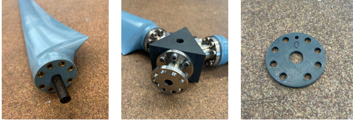
(a) Blade root with carbon rod extension.
