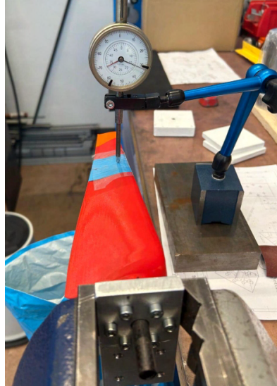
Figure 4.20: Experimental setup blade deformation test.
