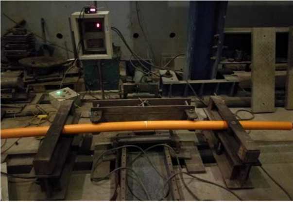
Figure 4. The four-point facility.
