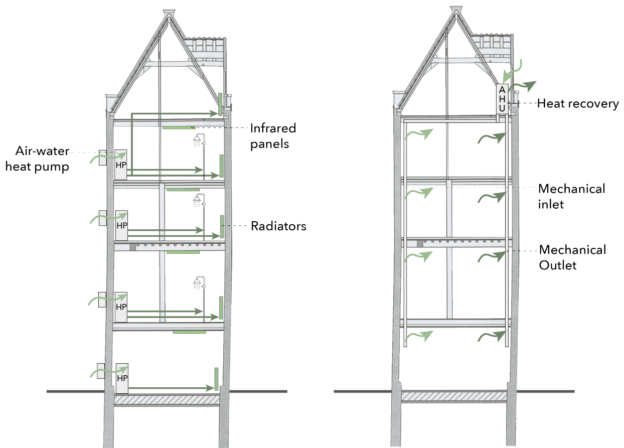
Figure 35: Heating & ventilation concept 2. Own work
