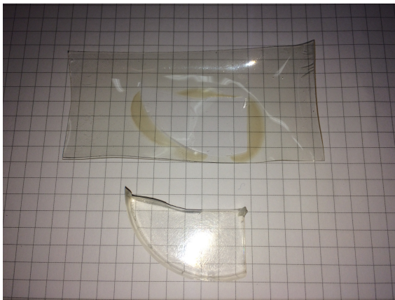
(a) Oxygen plasma etch of Topas® (Tg=70 °C), 99W, 30 min
