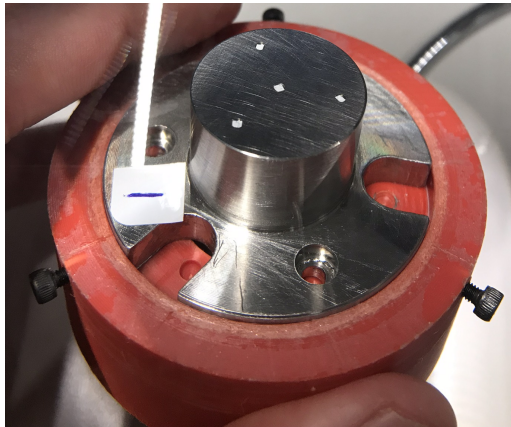
(a) The bearing inside a nylon holder to enable spin coating.
