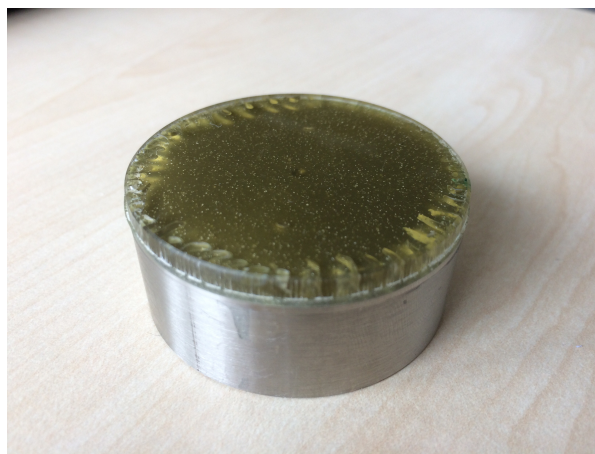
Figure E.27: Steel-Topas configuration with adhesive layer
