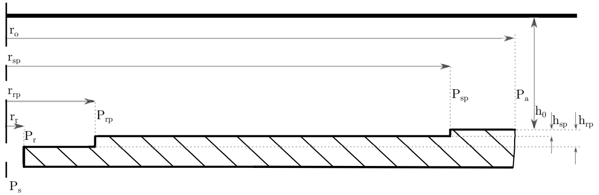
Figure 2.8: Axisymmetric bearing design with dimensions and local (nodal) pressures.
