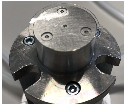
(b) The soft PDMS mask with holes at the shallow pocket positions.
