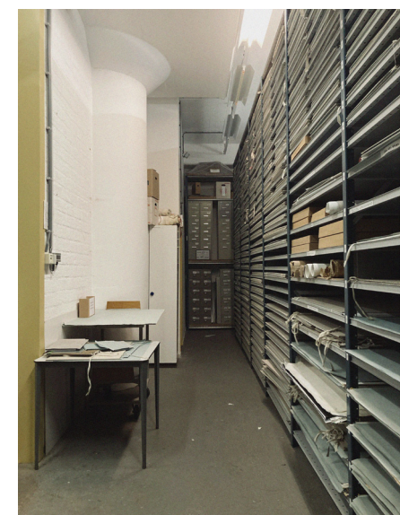
Fig. 10 Interior of the depot section of the IISH with the existing mushroom head concrete columns retained and plastered.
