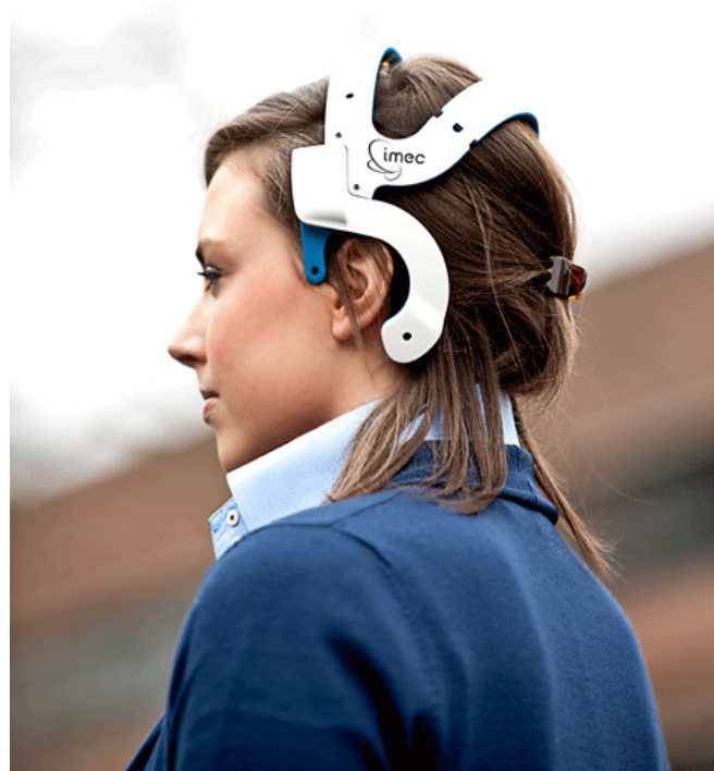
Fig. 1. IMEC's dry electrode headset for EEG monitoring.
