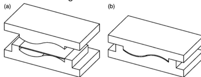
Figure 8. Illustration of matched die forming for a sheet in unloaded position (a) and in loaded position (b).
