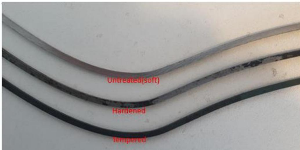
**Figure B.5.** Result of an untreated, hardened (quenched) and tempered beam.
