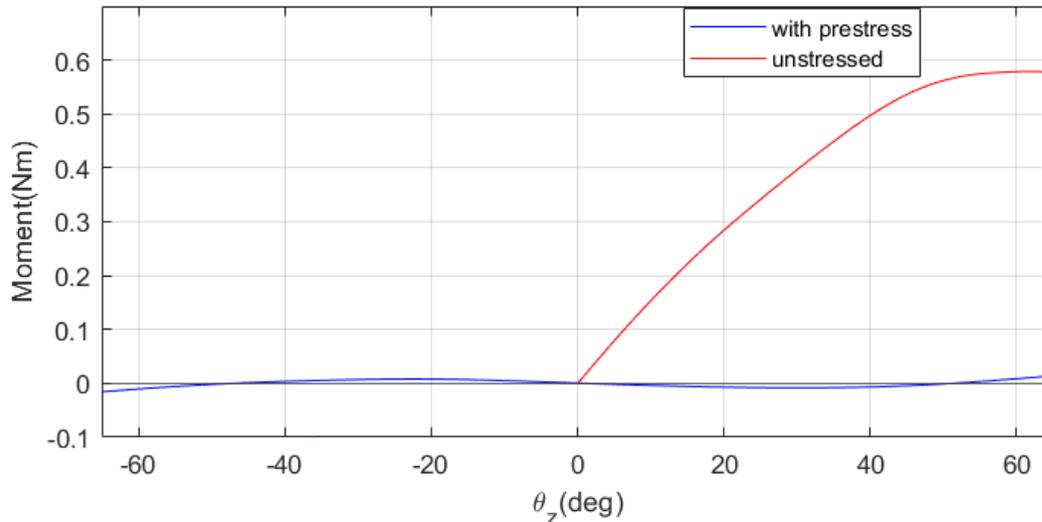
**Figure 21.** *The moment-angle curve of the unstressed and prestressed state of the compliant mechanism.*
