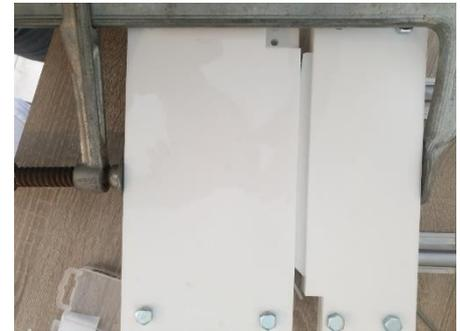
**Figure 15.** The setup of the bending tool where a glue clamp is used to press both parts together.
