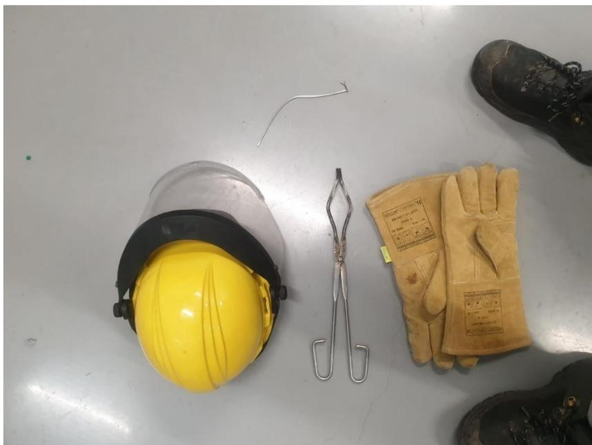
**Figure B.3.** Safety gear and gripper used to perform the heat treatments
