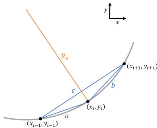
**Figure 9.** Schematic of a circle with radius of curvature  $R_o$  that goes through nodes  $P(i-1)$ ,  $P(i)$  and  $P(i+1)$ .
