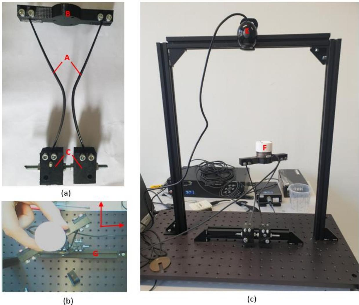
**Figure 16.** (a) Experimental setup of the mechanism where a camera is used to determine the angle of the connecting top body and a 6 DOF sensor is used to measure the applied moment when rotating the mechanism by hand. (b) The assembled mechanism. (c) A picture made by the webcam during an experiment.
