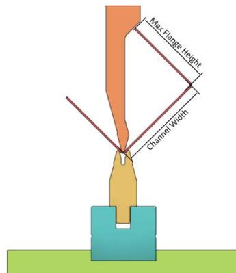
**Figure B.1.** *Illustration of the production of a U-beam with v-press braking*
