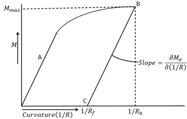
**Figure 10.** Relation between applied bending moment and curvature.
