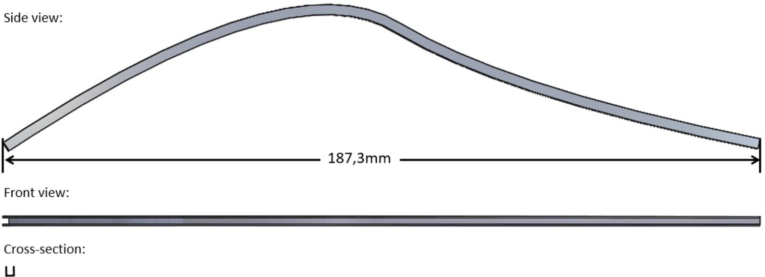
**Figure 3.** Side view, front view and cross section of the curved U-beam on scale 1:1
