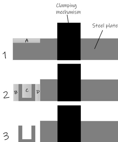
**Figure 6.** Steps of the milling process where a U-beam is milled from a metal plate. First part A is removed with an end mill cutter, and then parts B, C and D are removed with a slitting saw.
