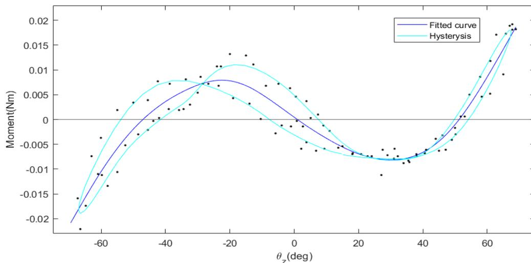
**Figure D.1.** The moment-angle curve of the experiment including the hysteresis and the black dotted data points
