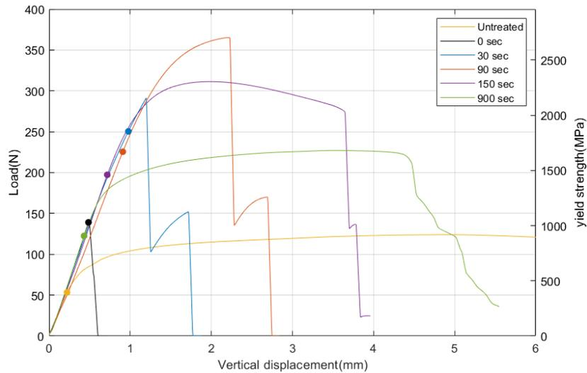
**Figure 19.** Load-displacement curve of a three-point bending test for 5 quenched steel U-beams with varying tempering times and an untreated steel U-beam.
