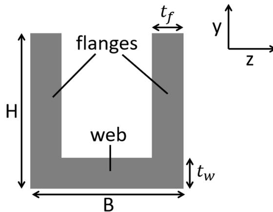
**Figure A.1.** Design parameters of the U cross-section
