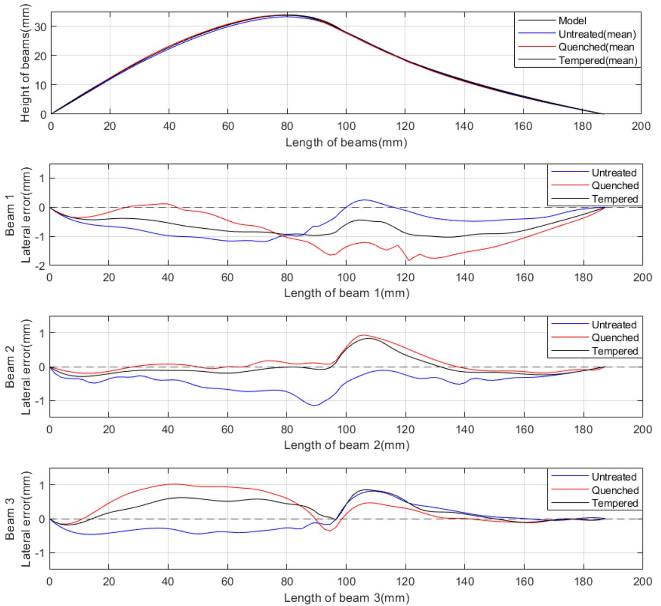
**Figure 20.** (a) The average curve of the three beams in untreated state, after quenching and after tempering of the quenched beam. (b-d) Lateral bending error of beam 1-3 for the three different states.
