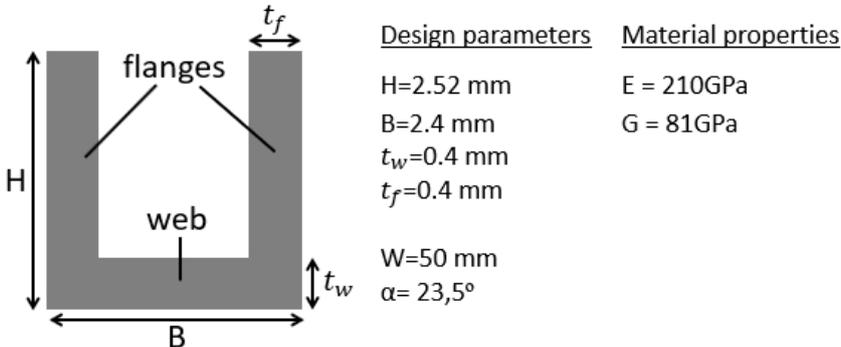
Figure 4: Design parameters of the design includes the dimensions of the U-cross section, the inclination angle  $\alpha$  and the leg width W. The material properties of steel used in the model are shown on the right.
