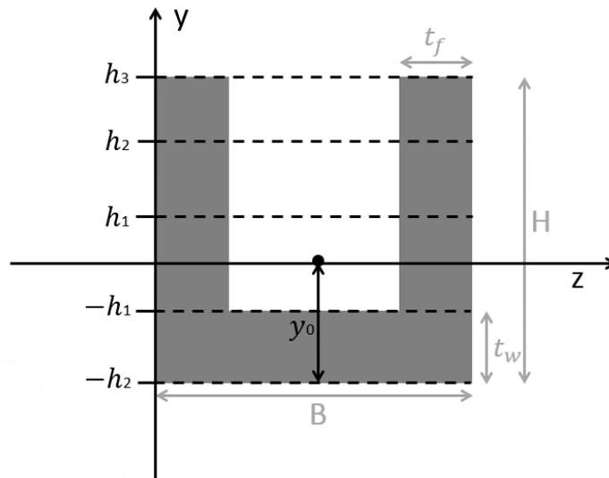
**Figure 11.** U-section of the beam where the  $z$ -axis is positioned at the neutral axis.
