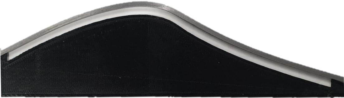
**Figure 17.** Result of a U-beam which is formed with the bending tool. The black mold shows the desired curvature at an offset of 5mm.
