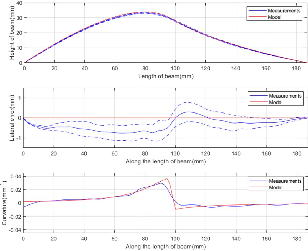
**Figure 18.** (a) Average curve of three beams with the standard deviation and the desired curvature. (b) Average lateral bending error of the three beams. (c) Comparison between the curvature of the produced beams and the model.
