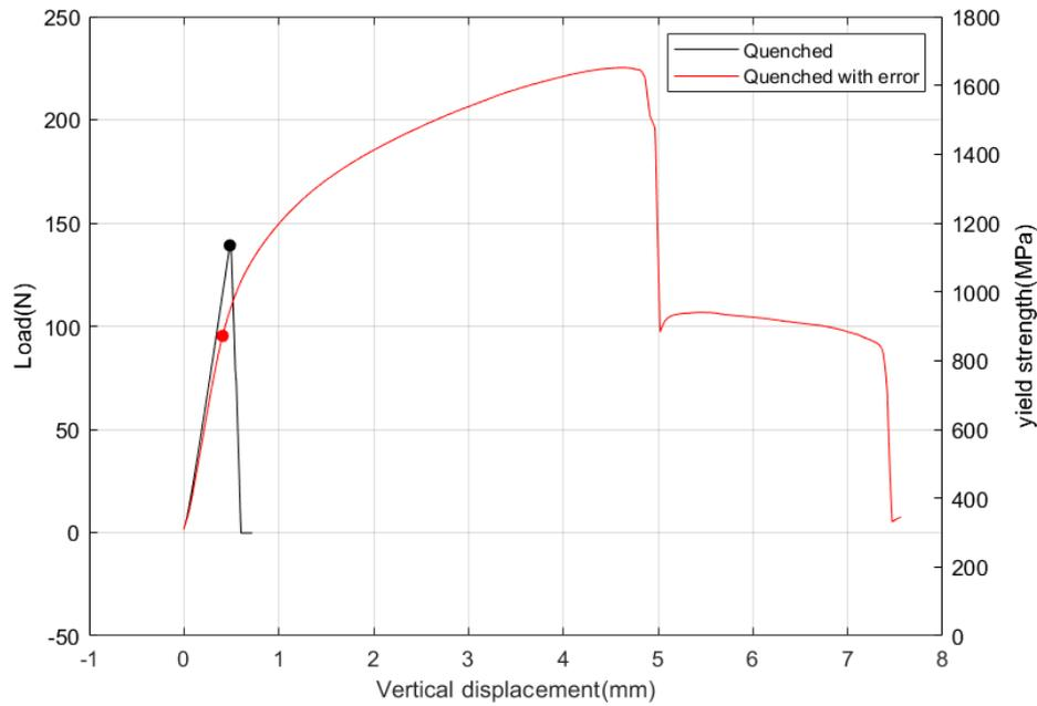
**Figure B.4.** Result of three-point bending test for a successfully quenched beam (about 0.5 sec in open air) and a beam which was in open air for a couple of seconds due to a human error.
