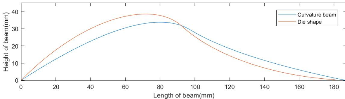
**Figure 13.** The calculated die shape using the 3 step method implemented in MATLAB.
