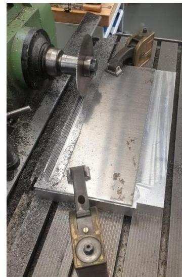
**Figure 7.** The setup of the milling machine where the steel plate is clamped to the bed with 2 clamping mechanisms.
