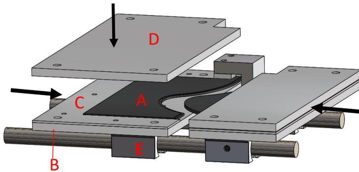
**Figure 14.** Design of the bending tool. The two matched dies are shown in black.
