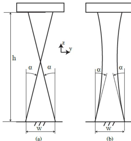
**Figure 2.** (a) Rear view of the undeformed beams and connecting upper body. (b) Prestress is applied by swapping the clamped ends of the beams, while holding the orientation of the connecting body, and without twisting the beams.
