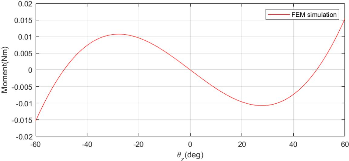
Figure 5. The moment characteristic of the rotational movement of the mechanism which is a result of a Finite Element Analyses.
