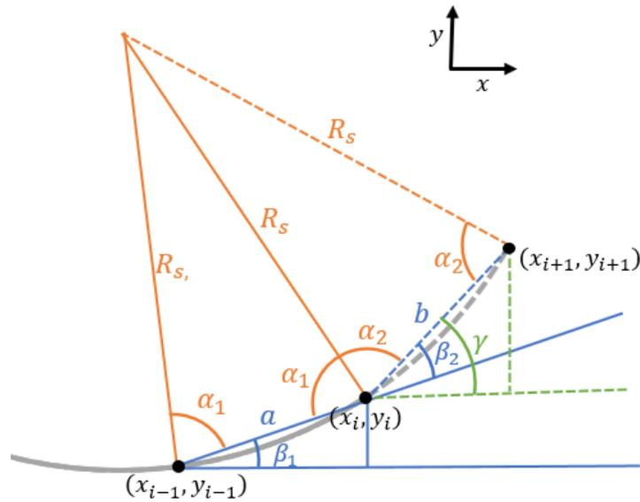
**Figure 12.** Schematic of the radius  $R_s$  of the circle that goes through nodes  $P(i - 1)$ ,  $P(i)$  and  $P(i + 1)$ .
