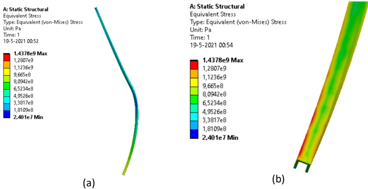
**Figure A.2.** (a) Ansys simulation of the U-beam in prestressed state. (b) Close up of bottom of the beam
