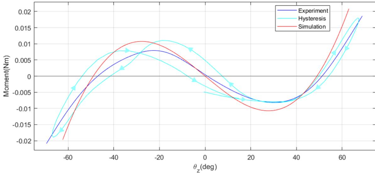
**Figure 22.** The moment-angle curve of the experiment including the hysteresis. Also, the predicted curve of the simulation is shown.
