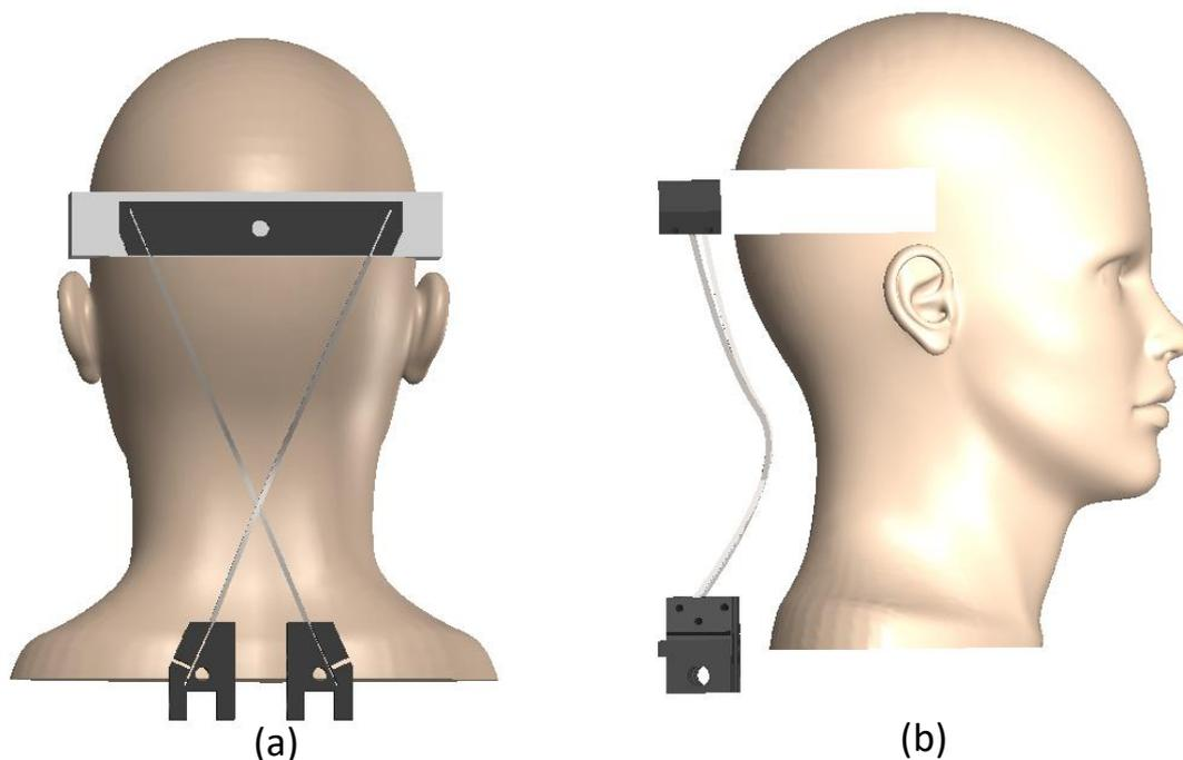
**Figure 1.** Design of the zero-stiffness compliant mechanism as a head support in unstressed state with:(a) Back view and (b) Side view
