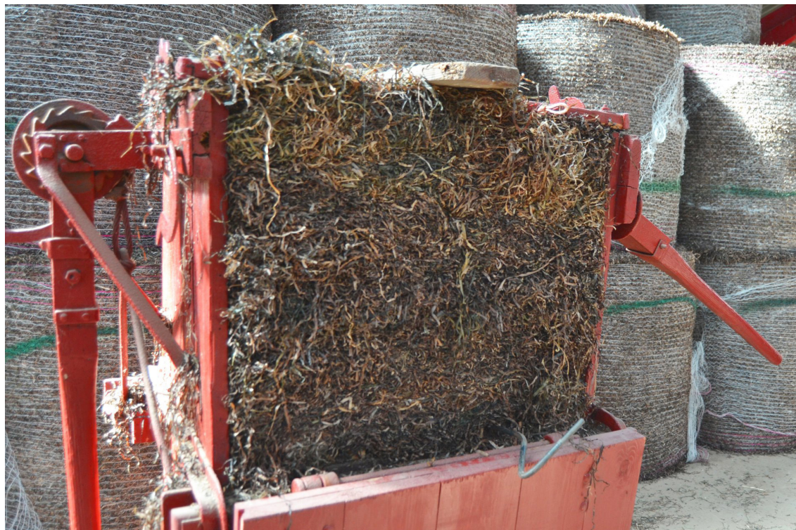
Fig 2: traditional Danish "seaweed farmer", Kurt Schierup from Møn Tang, processes dry eelgrass into bales for construction. Eelgrass is a type of seagrass native to the northern hemisphere.
