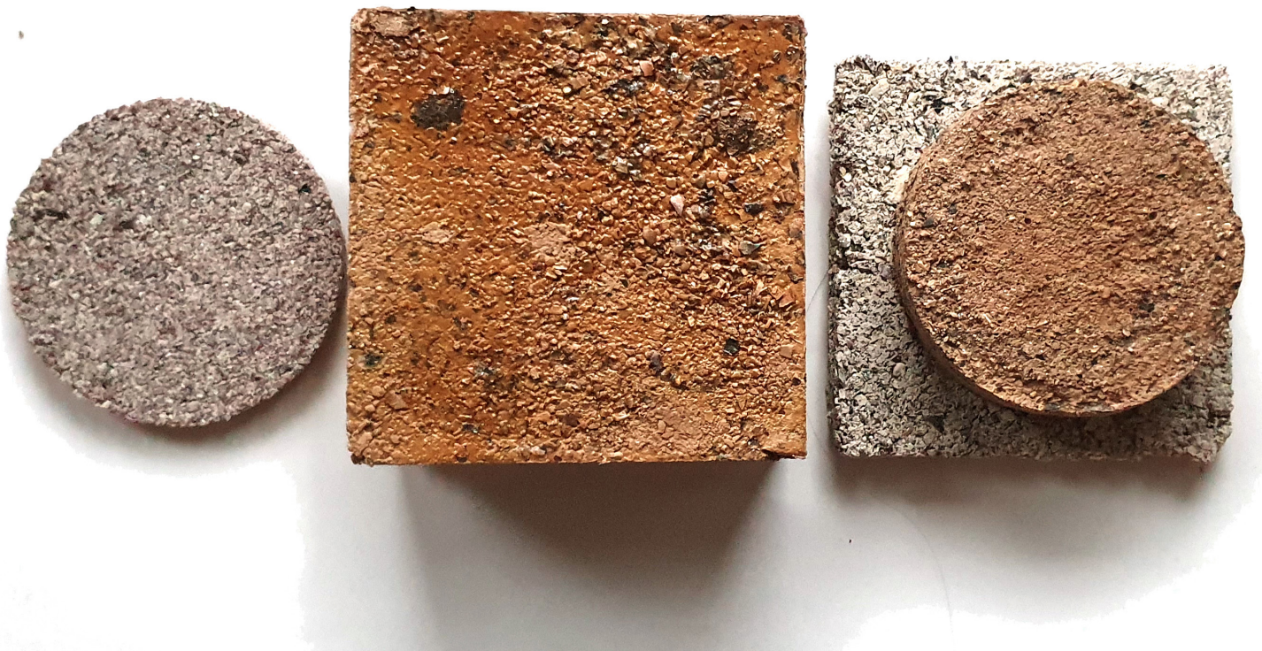
Fig 8: Shellcrete samples, made from mussel shells and cockle shells. Note the color difference between the white mussel shellcrete and the brown cockleshellcrete
