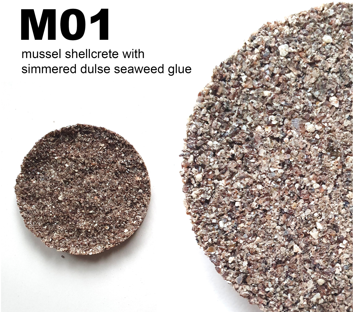
Fig 10: M01 Shellcrete Test
