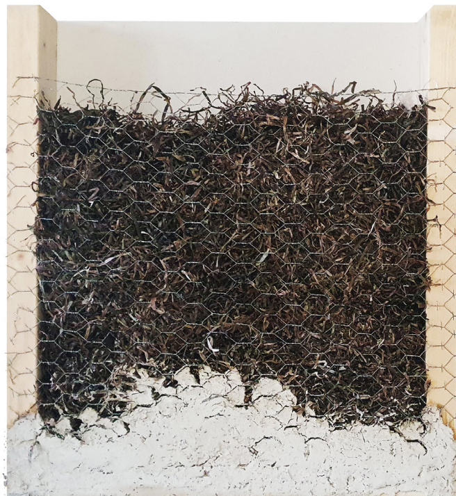
Fig 18: Top: Sargassum plaster with seaweed glue on fermacell board Bottom: Sargassum plaster with seaweed glue on chicken wire mesh over seagrass
