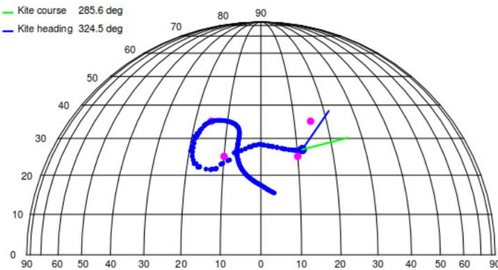
Figure 3.15: N-point tested using the backup link (biquad antenna, 10 Hz update rate,  $p_{loss} = 5.8\%$ ).
