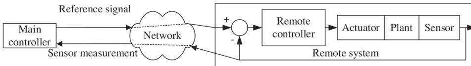
Figure 2.2: Hierarchical control system.
