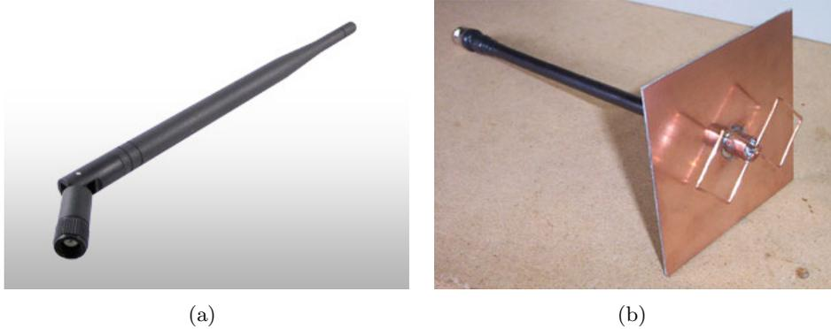
Figure 3.10: Dipole (left), and Biquad (right) antennas.
