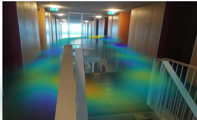
Fig. 1. Estimated magnetic field norm indoors from measurements from foot-mounted sensor.
