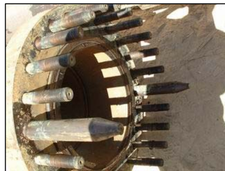
Figure 36 - Detail of drill-pipe flanges and connection bolts. To transmit the drill torque and carry the weight of pipes and cutterhead they are thick and are made from high-grade steel.
