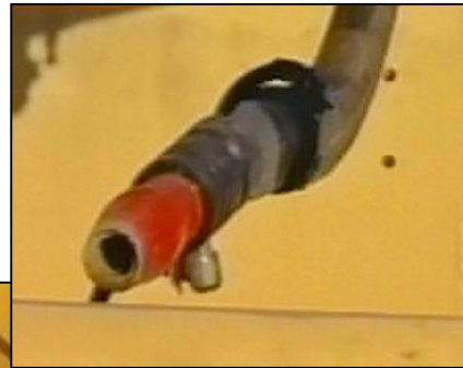
Figure 26 - Detail of fibrecrete nozzle
