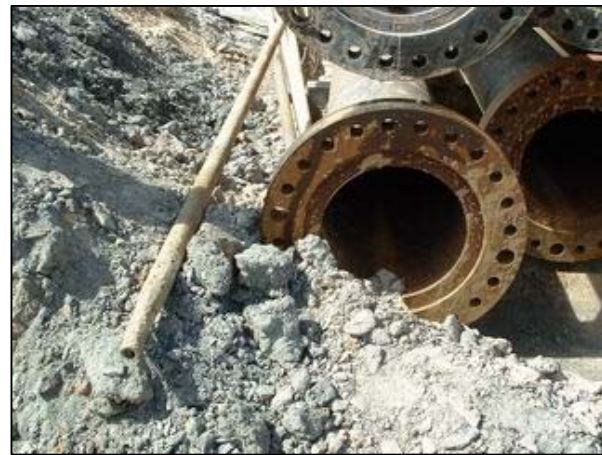
Figure 35 - Drill pipes and the airline-nozzle [left] which is lowered through the pipes.
