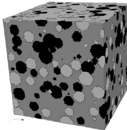
**Figure 1.** Computer generated microstructure of Gilsocarbon graphite, with filler particles in light grey and large pores in black (20%). Mass loss is simulated by "weakening" the matrix to match the mass loss.
