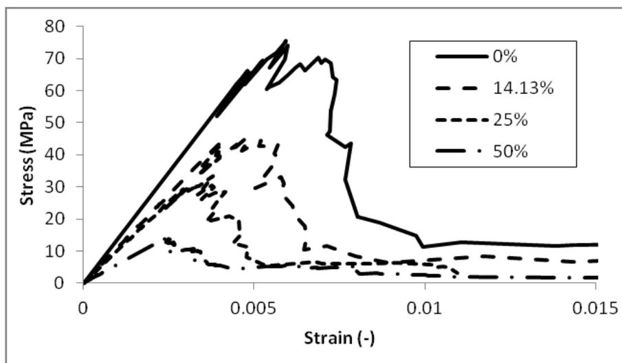
**Figure 3.** Simulated stress strain curves for Gilsocarbon graphite with increasing levels of irradiation damage (legend denotes weight loss).
