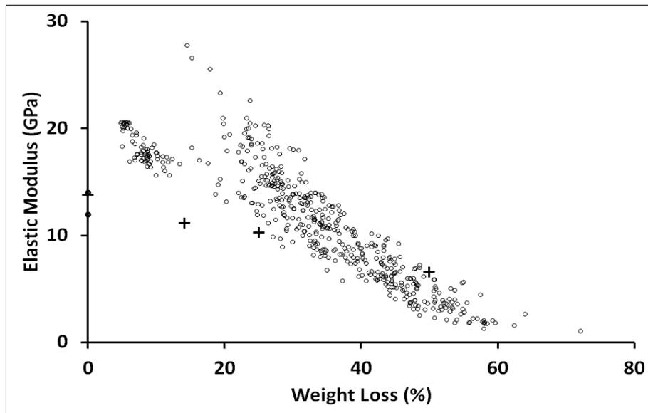
**Figure 4.** Comparison of the simulated (cross) and experimental (circle) values of Young's modulus for increasing weight loss.
