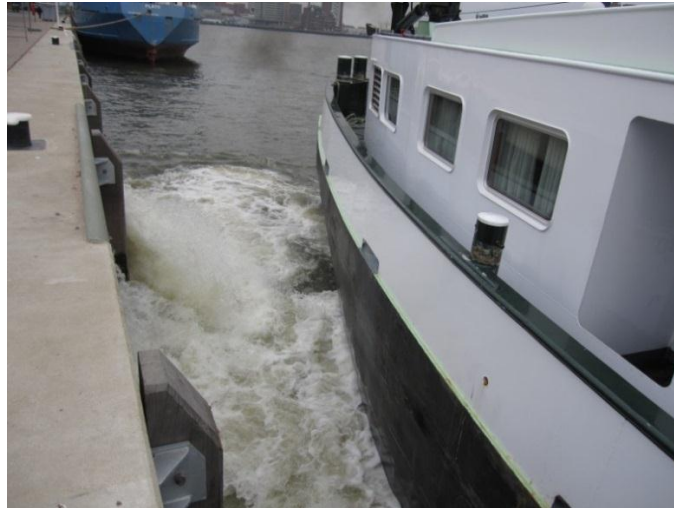
Figure B.3 Turbulent flow induced by main propeller
