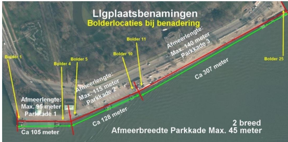
Figure B.6 The Parkkade in the Port of Rotterdam with approximate bollard location
