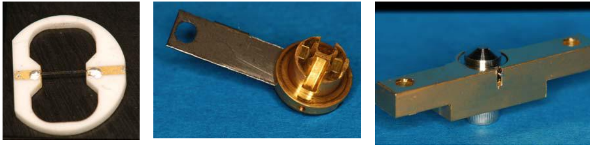
Figure 4 Left: Alumina device mounting ring with a SIS device mounted with two dots of silver epoxy. Middle: device mount with alignment spring attached. The heater is mounted in the backside of the device mount. Right: The pressure unit that pushes the device mount against the horn. The bullet-like part is pushed forward with an (internal) stack of spring washers.
