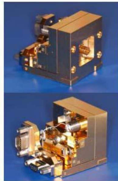
Figure 1 Left: Exploded view of the mixer block. Right: Front and backside view of an assembled mixer unit
