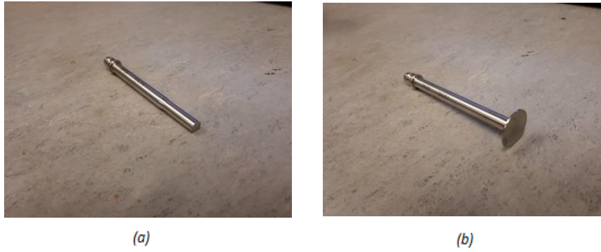
Figure 3.16: (a) 8 mm-diameter oscillating plate. (b) 25 mm-diameter oscillating plate.
