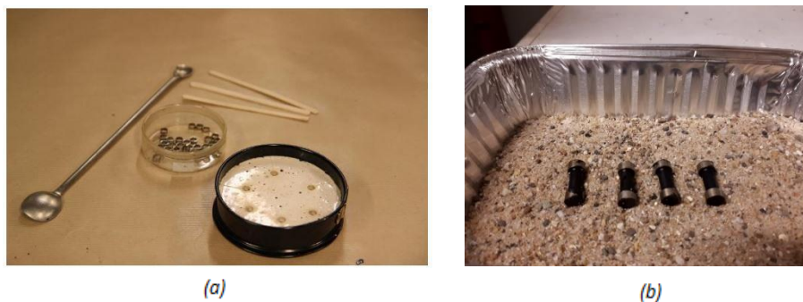
Figure 3.25: (a) Mastic column silicon mold. (b) Mastic column specimens.
