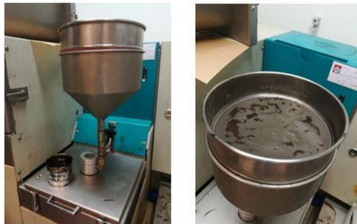
Figure 6.3: Removal of mineral filler particles larger than 63 \mu\text{m} .
