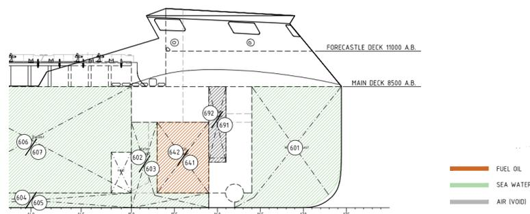
Figure 3.3: Fore side view of storage tanks
