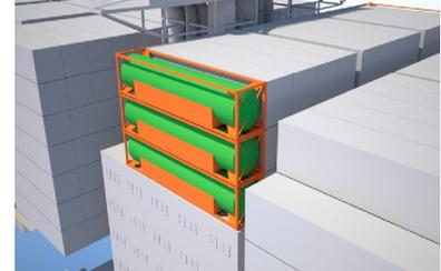
Figure 4.6: Portable fuel tank [45]
