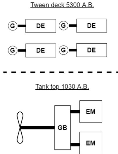
Figure 3.6: Schematic diesel-electric power plant layout
