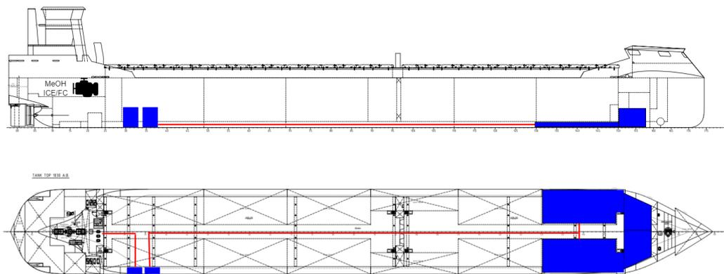
Figure 4.10: General arrangement drawings of concept design 1 with methanol storage
