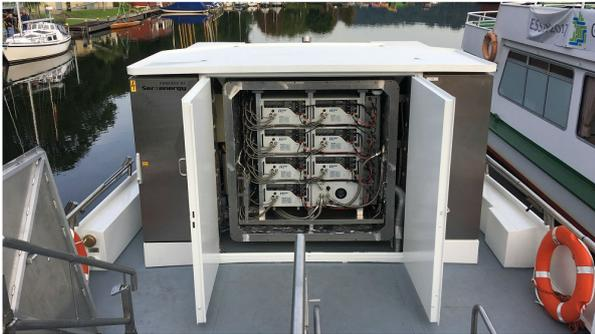
Figure 4.20: HT-PEMFC units on board of MS Innogy (35 kW) [89]
