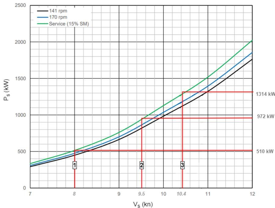
Figure 3.10: Power-speed curve
