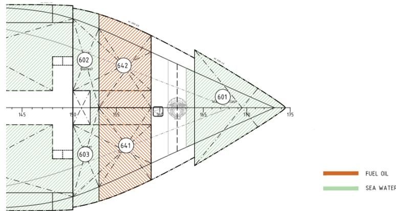
Figure 3.4: Fore top view of storage tanks
