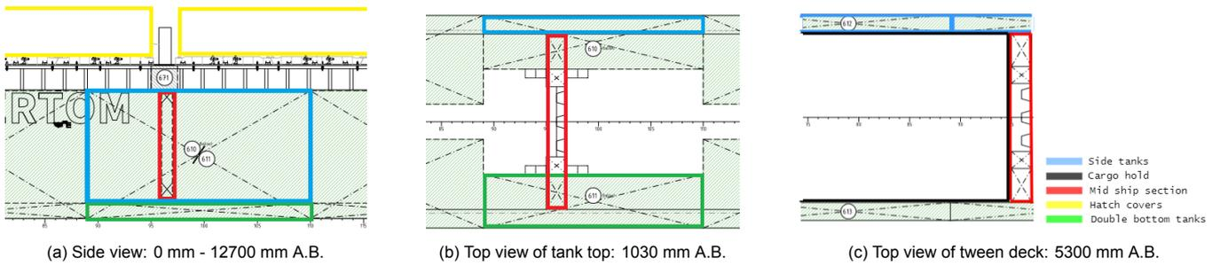
Figure 4.8: Potential spaces to store methanol in mid ship
