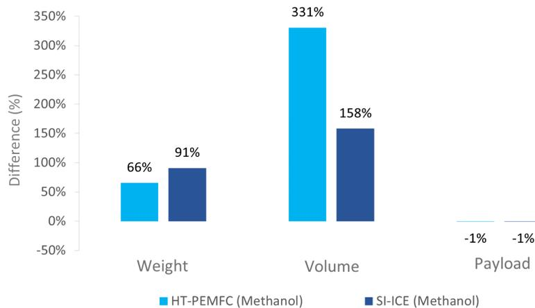
Figure 4.23: Weight and volume comparison of methanol power- and energy systems with respect to a diesel power- and energy system
