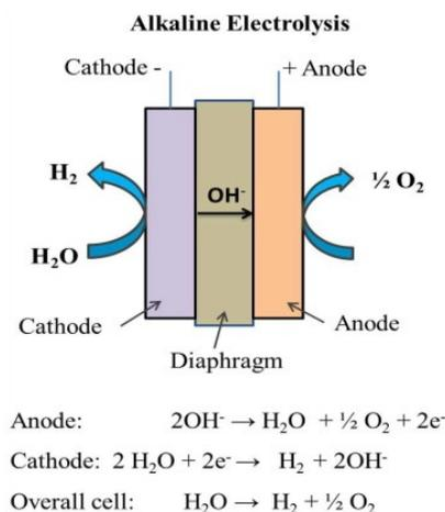
Figure 2.6: Schematic process of an alkine electrolyzer [85]
