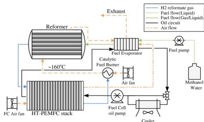
Figure 4.18: Schematic representation of a methanol HT-PEMFC power plant [86]
