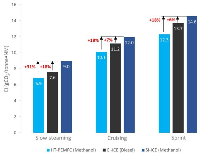
Figure 4.26: Emission index (EI) comparison per operational mode between the current diesel configuration (CI-ICE) and future methanol configurations (HT-PEMFC and SI-ICE)
