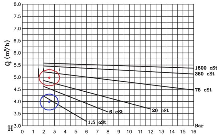
Figure A.1: Operation point (Red = MGO, Blue = Methanol)
