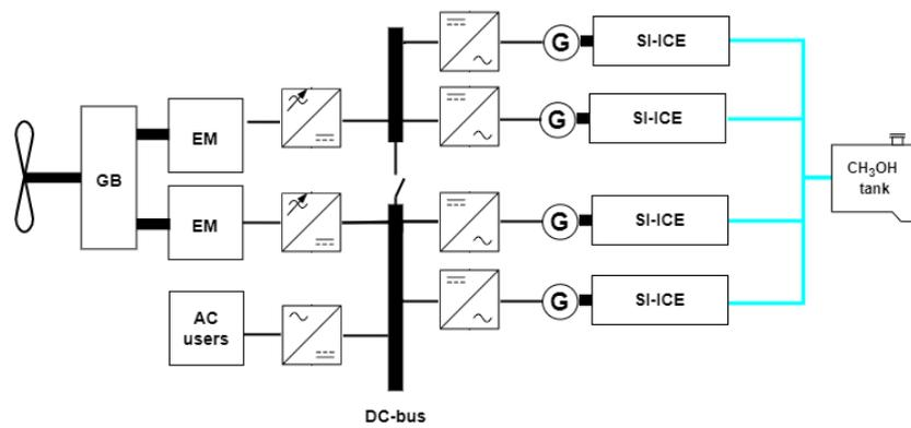
(a) Power plant layout with an SI-ICE on methanol
