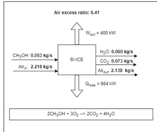
Figure 4.16: Mass- and heat balance of a 400 kW methanol SI-ICE
