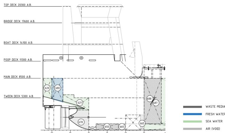
Figure 3.5: Aft side view of storage tanks
