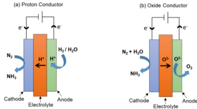
Figure 2.13: Solid state ammonia synthesizer [33]
