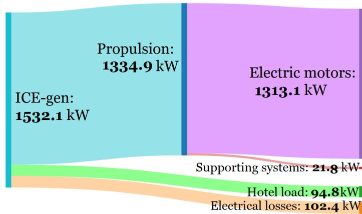
Figure 4.17: Sankey diagram of the electrical load for winter sailing for an SI-ICE power plant
