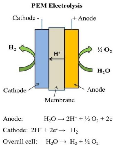
Figure 2.8: Schematic process of PEM electrolysis [85]
