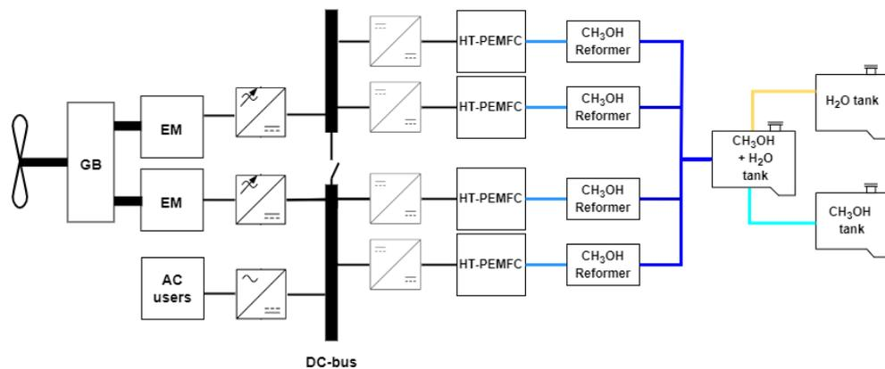
(b) Power plant layout with a PEMFC on methanol
