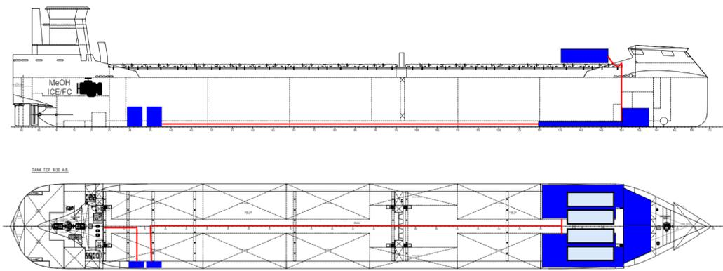
Figure 4.12: General arrangement drawings of concept design 3 with methanol storage
