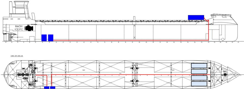
Figure 4.11: General arrangement drawings of concept design 2 with methanol storage
