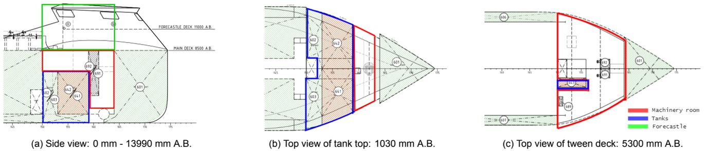
Figure 4.7: Potential spaces to store methanol in fore ship
