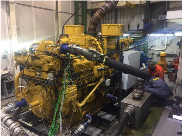
Figure 4.15: Setup of a CAT G3508A on methanol [9]
