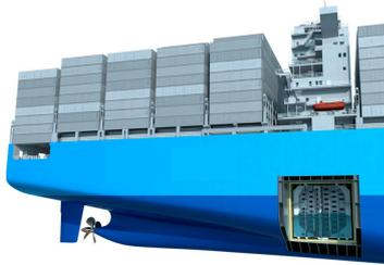
Figure 4.4: Integrated fuel tank [54]
