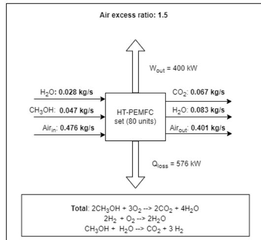
Figure 4.21: Energy flow balance of a 400 kW methanol HT-PEMFC set
