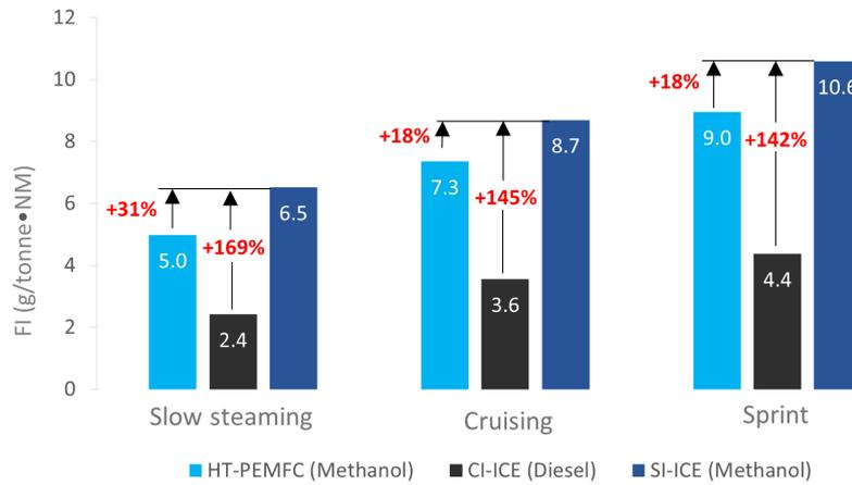
Figure 4.24: Fuel index (FI) comparison per operational mode between the current power- and energy system (CI-ICE) and future power- and energy system (HT-PEMFC and SI-ICE)
