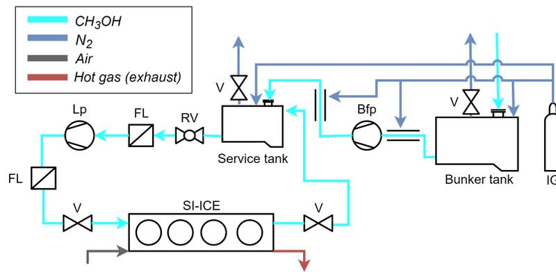
Figure 4.14: Layout of a 100% methanol fuel system with a SI-ICE
