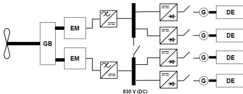
Figure 3.7: Power plant layout with part of electric system
