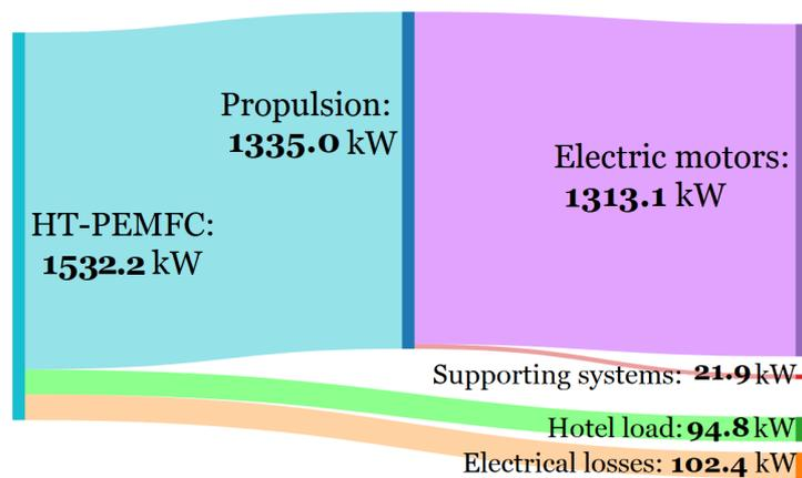
Figure 4.22: Sankey diagram of the electrical load for winter sailing for an HT-PEMFC power plant
