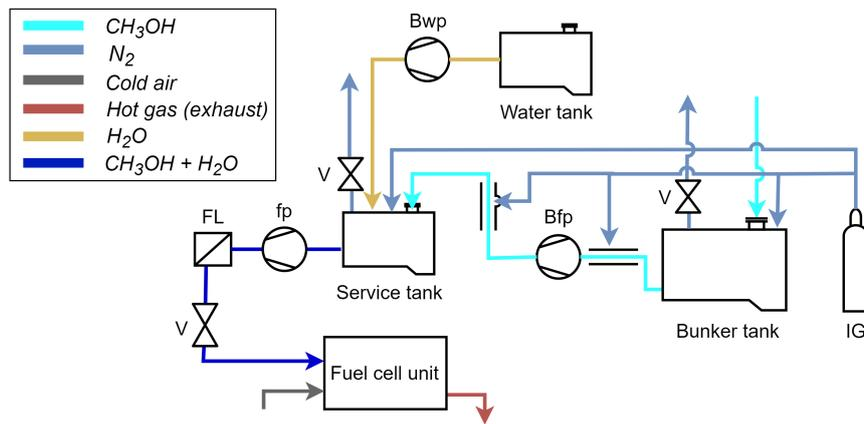
Figure 4.19: Layout of a methanol fuel system with a HT-PEMFC unit
