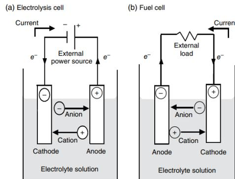
Figure 4.1: Working principle of an electrolyzer and fuel cell [18]
