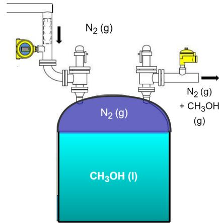
Figure 4.3: Methanol storage tank with inert gas system [4]
