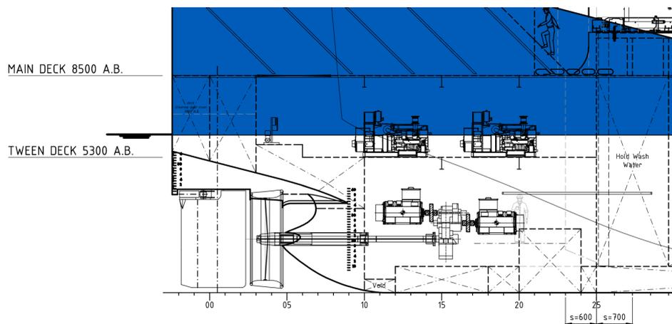
Figure 3.1: Side view of the propulsion- and engine room
