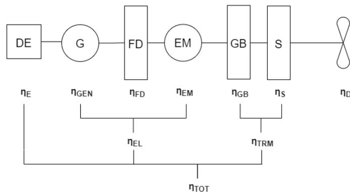
Figure 3.9: Power train of the propulsion
