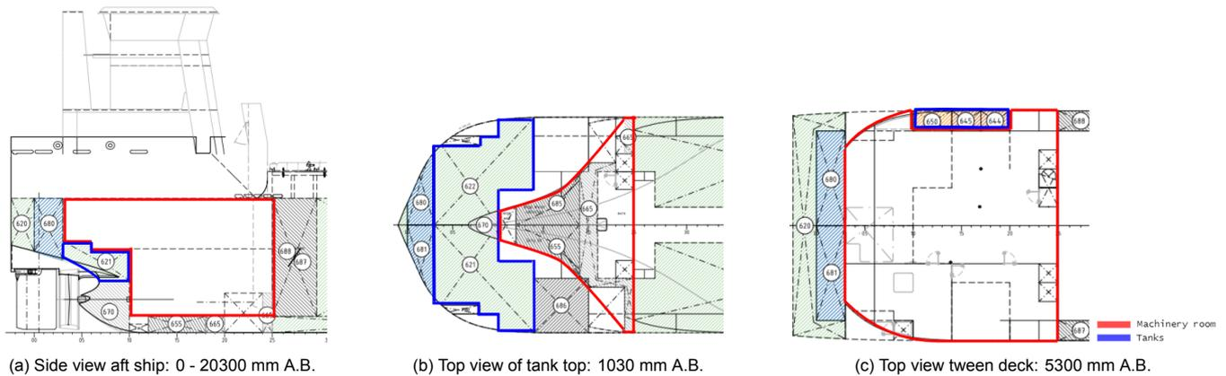
Figure 4.9: Spaces for methanol storage in aft ship
