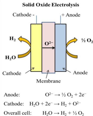
Figure 2.7: Schematic process of solid oxide electrolysis [85]
