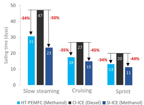
Figure 4.28: Operational time comparison per operational mode
