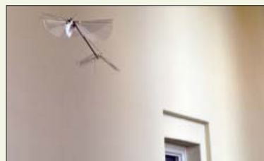
The DelFly passing through a corridor. The two pairs of interconnected wings are flapping at about 6 hertz.
