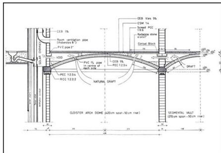
111. Ventilation system through the vaulted structures towards the solar chimney. Source: AurovilleEarthInstitute
