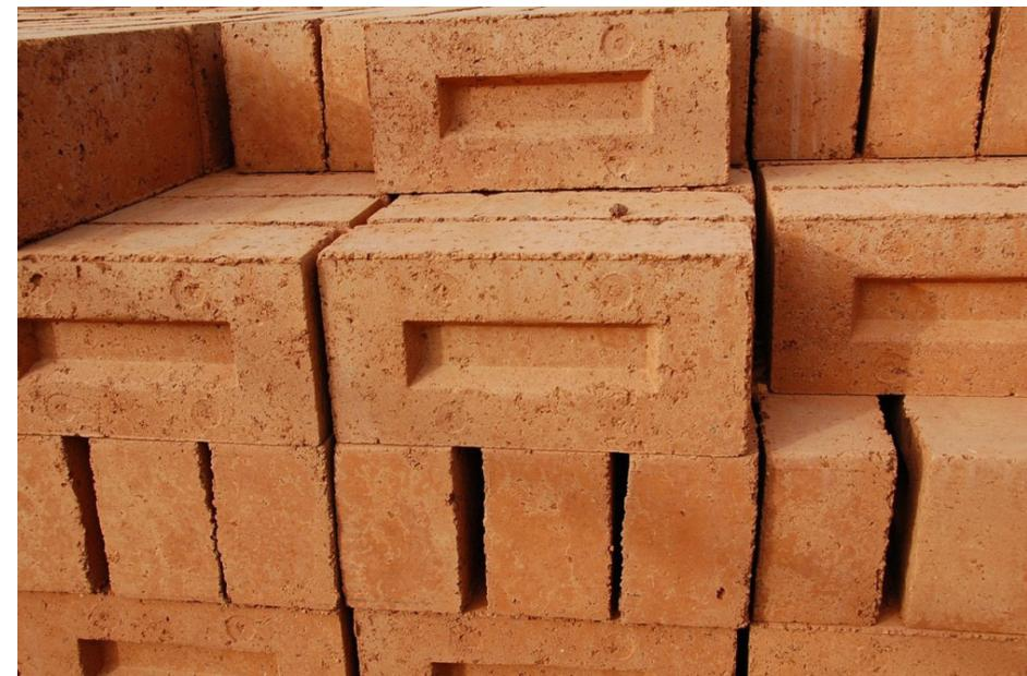
107. Compressed Earth Block. Source: Structural guide, Kalkionline, 2024
