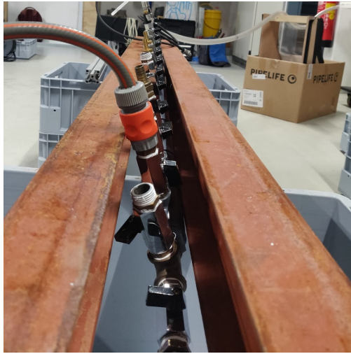
Figure C.1: Calibration setup for the pressure sensors. A long PVC pipe with several fittings to connect the pressure sensors. A garden hose is used to pump water into the system. On the upper right of the figure a white hose is visible. This hose extends upwards, approximately 10 m of water column can be applied to the sensors.
