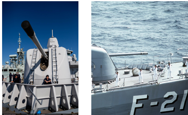
Figure 2.1: Two examples of breakwaters on navy frigates. (a) Vertical breakwater on Dutch frigate Zr. Ms. Evertsen [11]. (b) Forward tilted breakwater on Venezuelan frigate ARV Mariscal Sucre [34].
