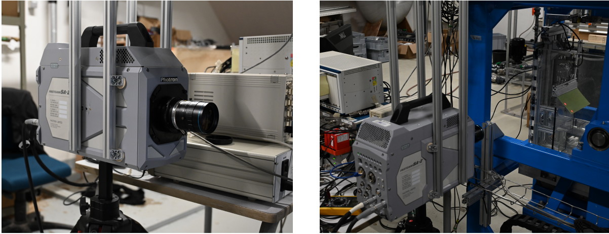
Figure 2.8: The high speed camera that was used during the experiments (a) Front view of the camera, with the frame keeping it in place. (b) Rear view of the camera, with a view on the test setup.
