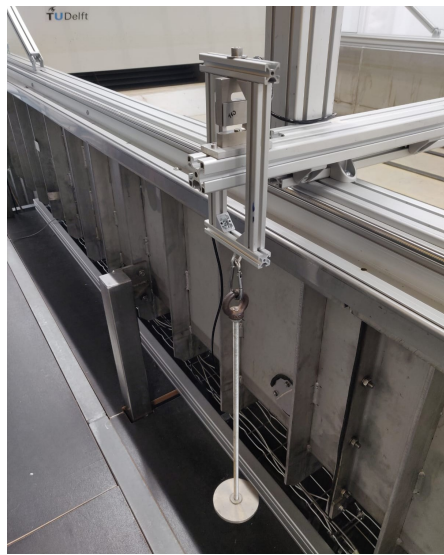
Figure C.5: Calibration process of the load cells. (a) Separately, outside of the setup. Calibration in compression, tension was also applied. (b) In the test setup. Only compression was applied, the load cells were also loaded in compression during the wave impacts.
