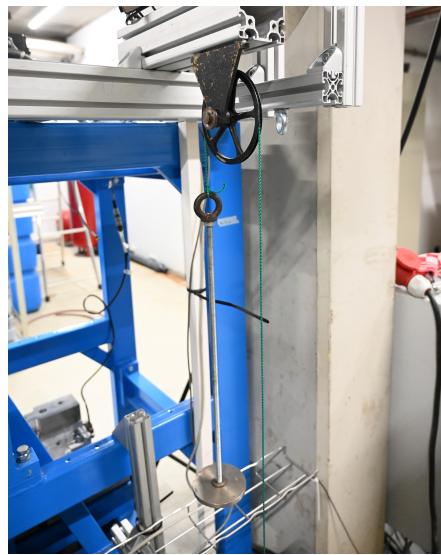
Figure C.5: Calibration process of the load cells. (a) Separately, outside of the setup. Calibration in compression, tension was also applied. (b) In the test setup. Only compression was applied, the load cells were also loaded in compression during the wave impacts.
