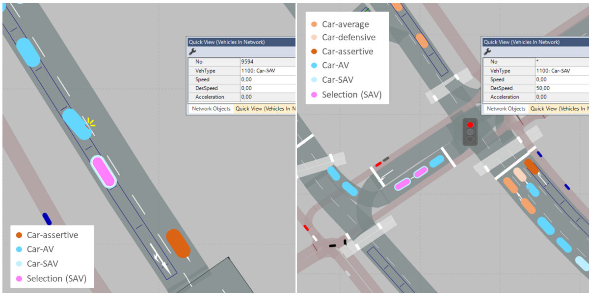
(a) Bottleneck created by SAV (b) SAVs using a low capacity link
