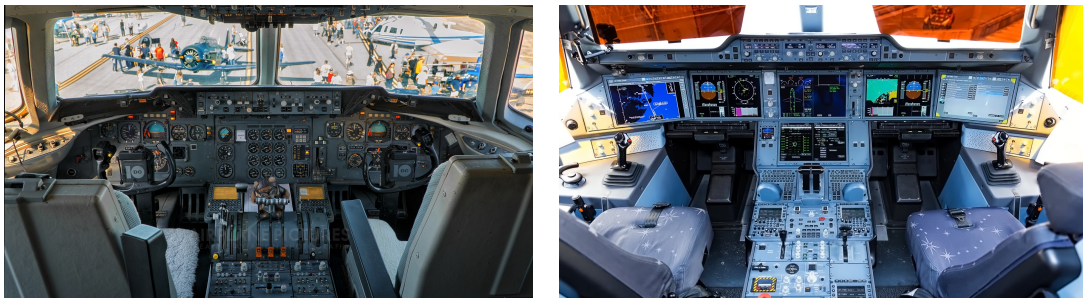
(a) Classic flight deck on the McDonnell Douglas DC-10. (b) Modern flight deck on the Airbus A350.
