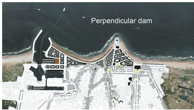
Figure 6. Scenario 'City in the sea', in which the urban fabric slowly grows seawards around a perpendicular dam where sedimentation takes place and building land emerges. Source: Atelier Kustkwaliteit (2011), Werkboek #1, edited by authors.
