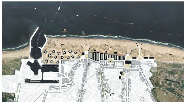
Figure 8. (right): Scenario 'Soft seaward' works with a new stretch of dunes that creates a natural environment for a more nature-sensitive form of development. Source: Atelier Kustkwaliteit (2011), Werkboek #1.
