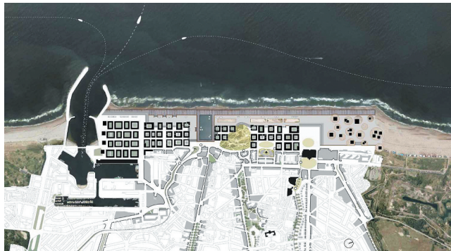
Figure 7. (left): Scenario 'Hard seaward' projects the water barrier on the edge of land and sea, which makes it possible to build new urban fabric behind it. Source: Atelier Kustkwaliteit (2011), Werkboek #1.
