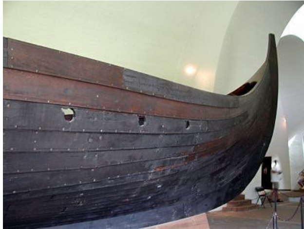
Figure 5.23 Wooden splines on the hull of a Viking ship. (Source: Oslo Viking Ship Museum)
