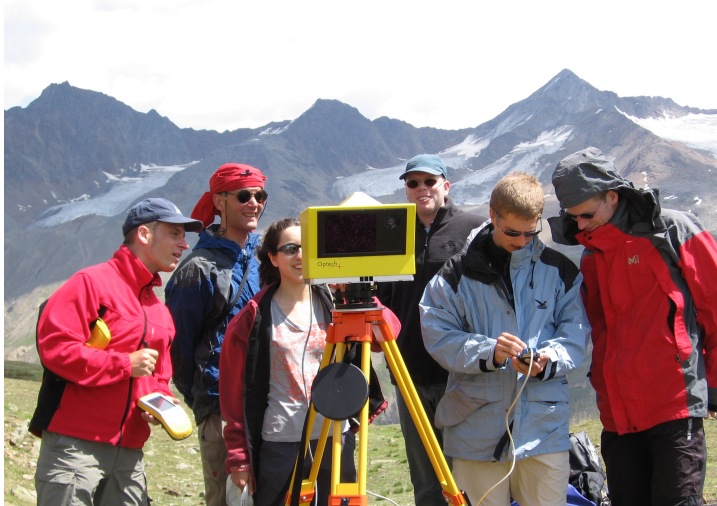
Figure 3.11 Expedition to the Hintereisferner. Expedition members and ILRIS 3D Terrestrial Laser Scanner.
