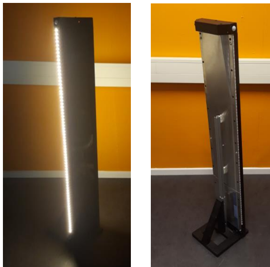
Figure 12: A front (left) and back (right) image of the final version of the indoor PV lamp.
