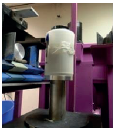
Figure 5. The 738 g sample being counted after neutron activation
