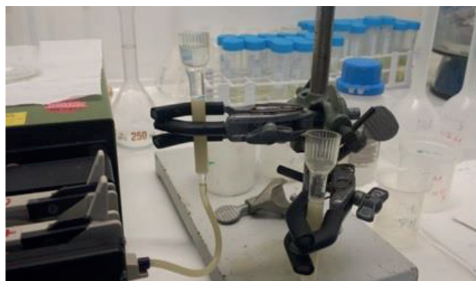
Figure 1 Bio-Rad Poly-Prep column filled with 2 ml of the strong anion exchange resin AG 1-X8 (100-200 mesh).
