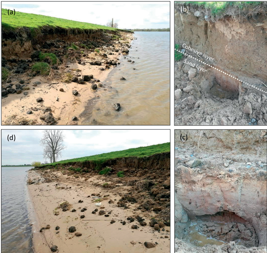
Figure 5.7. (a) Downstream view of the left bank at Neerloon, with cohesive slump blocks over a sandy terrace (April 5, 2019). (b) Composite structure with transition at the upper-bank toe. (c) Lower sand layer collapsing by own weight at same location, after few minutes of excavation. (d) Upstream view of stretch with longer terrace than panel a) on same day.
