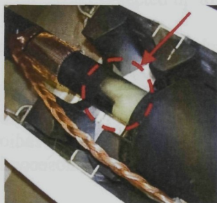
Figure 2.12: (left) Defect: Missing insulation screen at the cable/joint transition. (right) S/N of spectra measured at internal inductive sensor mounted close to the joint 33kV. Detection with an IEC 60270 system indicated 100pC.
