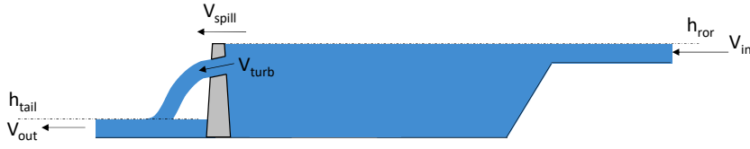
Figure 3.6: Schematic overview of a run of river node. The figure indicates the upstream and downstream head and the in and outgoing flows. Because the minimal storage of these plants is neglected, the inflow should be equal to the outflow.
