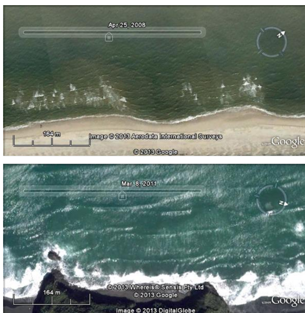
Figure 1.4: Examples of different sea states. Top panel shows an aerial photograph taken at the Dutch coast, showing short wave crests and short period waves. Bottom panel shows longcrested long period waves arriving at the coast of New Zealand. Both images are to similar scale. Image data: Google, Aerodata, DigitalGlobe.
