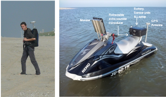
Figure A.1: Equipment used to survey the topography. Septentrio GPS backpack (left) and survey jetski NEMO (right).
