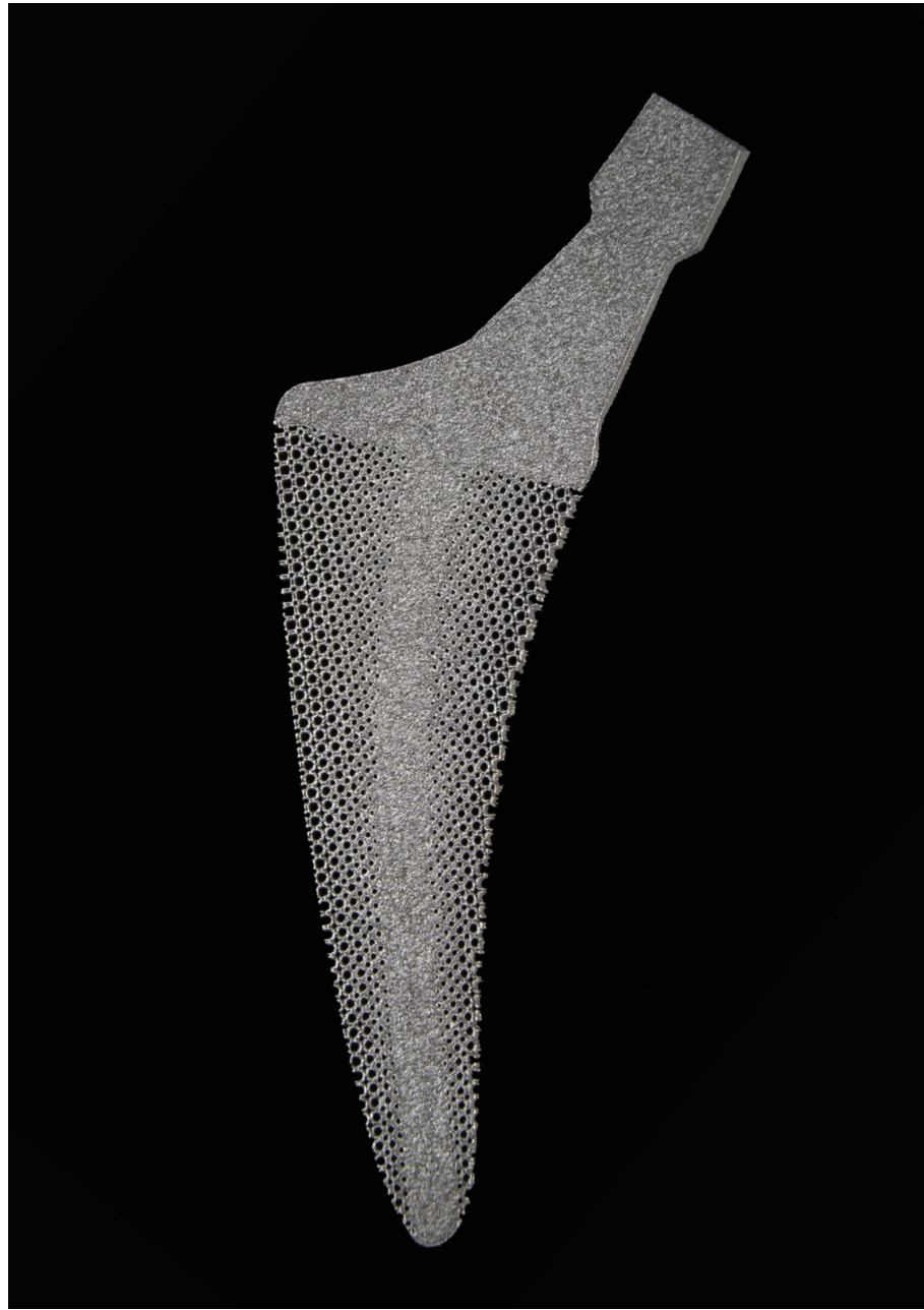
Figure 9.4: . Specimen fabricated using selective laser melting (SLM). Material: Ti-6Al-4V ELI (Extra Low Interstitials) ASTM B348 with a particle size range of 10-45 micron, Machine: GmbH SLM125
