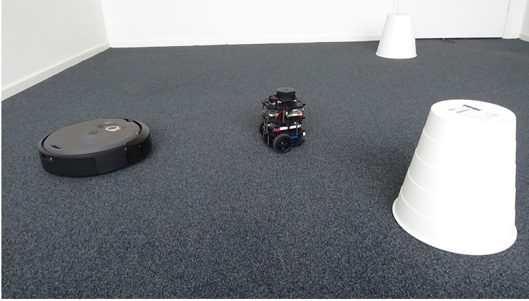
Figure 2.12: A view of the scenario of the experiments, with the robots (the TurtleBot used as the SaR robot is in the middle and the iCreate3 robot used as the victim is at the side) and the obstacles (white buckets).
