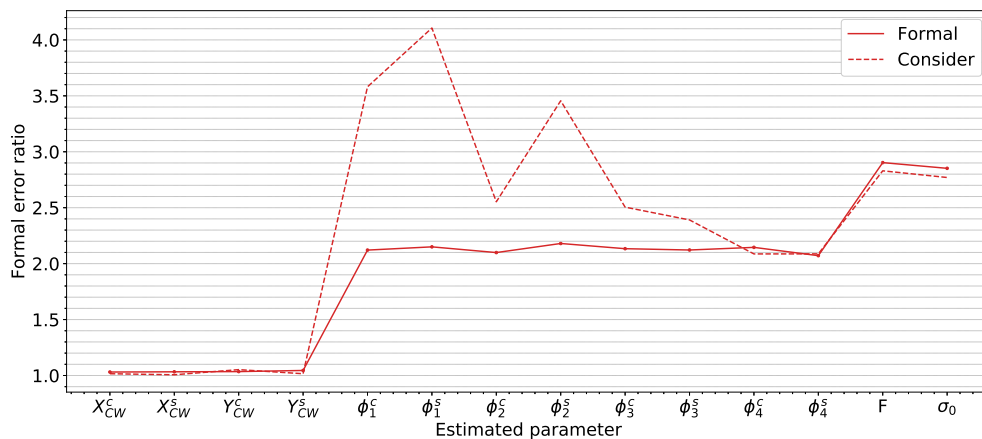
Figure 6.26: Uncertainties of the estimation case with arcs of 5 days relative to the nominal solution
