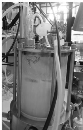
Figure S2.1. A. niger wall growth accumulation in the fermentor during fermentation (A) and before cleaning (B).
