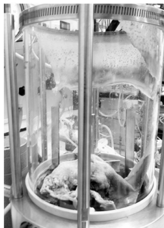
Figure S2.1. A. niger wall growth accumulation in the fermentor during fermentation (A) and before cleaning (B).
