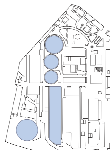
650 m Gasholder 1 175 x 35 m Bassin 400 m Gasholder 2,3 500 m Gasholder 4
