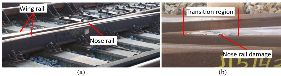
Figure 2. A 1:9 cast manganese steel crossing: (a) view of a wing rail and crossing nose rail, and (b) crossing nose rail damage in the transition region.
