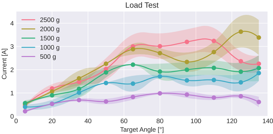
Fig. 4. Results of the static load test. The system is loaded in increments of 500 g, from 500 g to 2500 g. Mean values and the quadratic interpolation are presented with their standard deviation.
