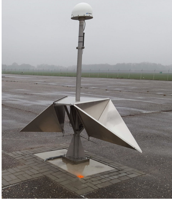
Fig. 2.10 Integrated Geodetic Reference Station (IGRS), design by Delft University of Technology
