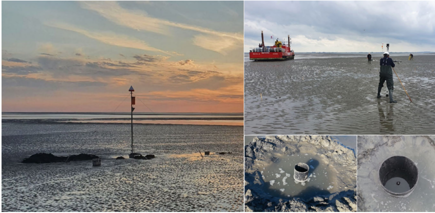
Fig. 2.5 GPS measurement setup in the Wadden Sea area. Mutual height differences between the (three) deeply founded benchmarks per cluster location are measured with leveling as well. Campaign GPS measurements are done over 5 d. The height of the GPS antenna is such that it stays above the water line at high tide
