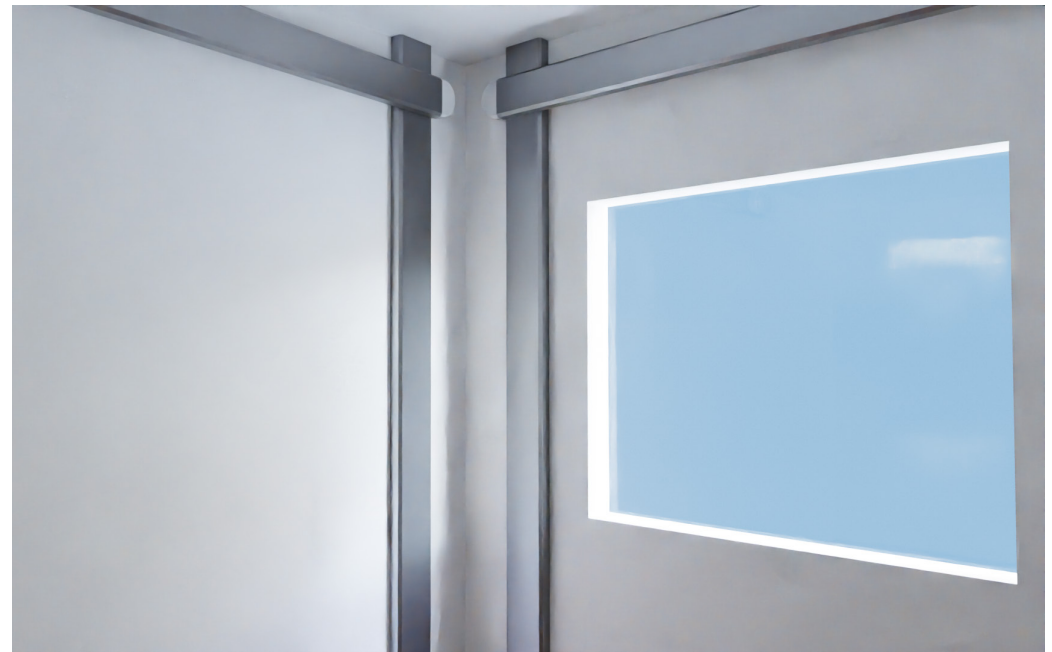
Figure 16: A render of a corner with both an exhaust and a supply riser.
