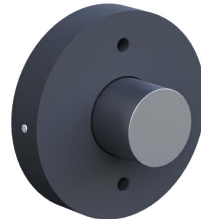
Figure 39: A visualisation of the full assembly of suspension parts. The rod in the middle would be fixed to the duct before assembly.
