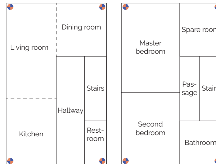
Figure 70: A blueprint with the riser locations.
