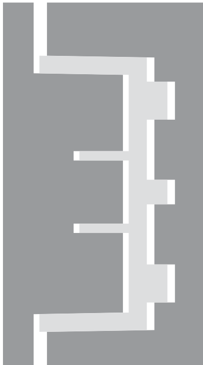
Figure 44: Simplified cross section of the molds of the main housing.
