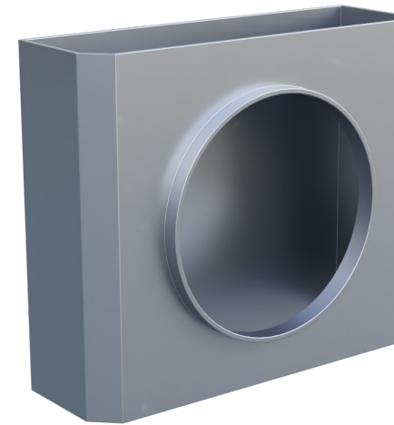
Figure 13: A preview of the riser to air duct connection part.
