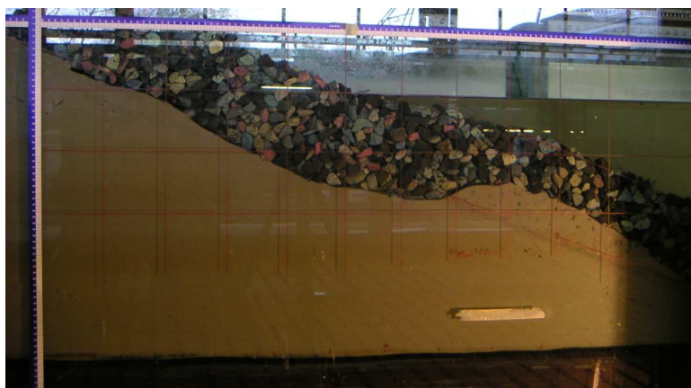
Figure 8 Photograph experiment 3 at start (a), 600 (b) & 2400 (c) waves
