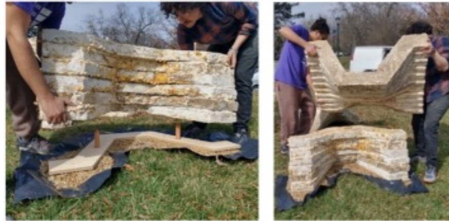
Serpentine wall study - assembling bio welded components, 1200mm tall
