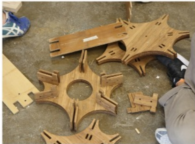
Assembly of CNC cut 8mm thick components
