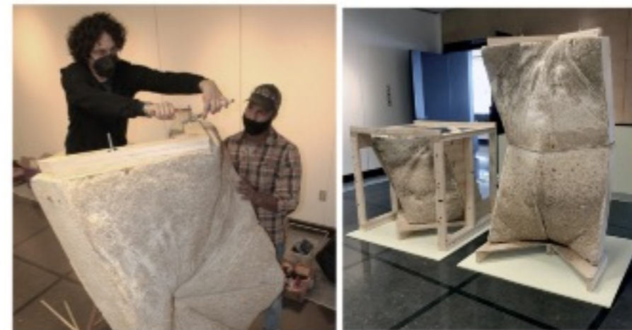
Post-tensioning the prototype - tightening the cables
