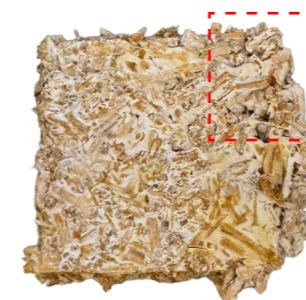
Disintegration at the corners
